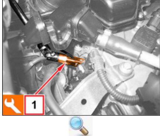
1. Undo and remove the UNIAIR module oil temperature sensor using the tool.
